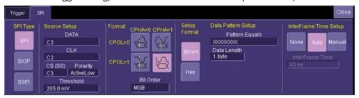
The SPIbus trigger dialog is very flat, meaning there are few dynamic changes to the dialog based on selections within. The one exception is the SPI Type on the far left. When selecting between SPI, SIOP, and SSPI types, the dialog to the right changes to reflect a specific setup type.
