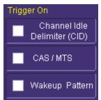
Include or exclude **Channel Idle Delimiter (CID)**, **CAS/MTS**, or **Wakeup Pattern** from your trigger by checking our un-checking as desired. Multiple values may be selected and included in your Symbol trigger.
