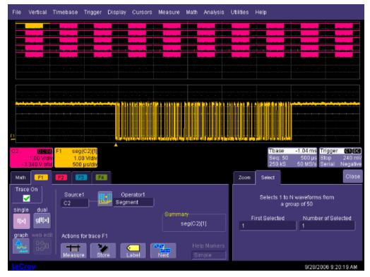
• You can view decoded data on the individual segment by setting up the Decode to use the Math trace as the source for Data (in this case F4 is the Source). If you wish to change the segment that is decoded, just select a new segment from the Math trace dialog (as shown in the previous step).
