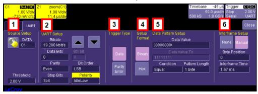
The previously numbered UARTbus trigger sections correspond with the following explanations.
