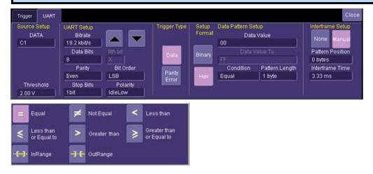
The Source and UARTbus Setup information must be defined. The datasheet for your part should contain the information you need to properly setup the UART Trigger.
