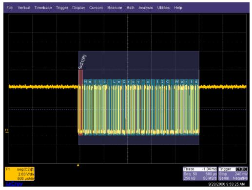
• You can view the timestamps for each segment by selecting **Vertical > Channels Status** from the menu bar and selecting **Time** on the **Show Status For** section of the dialog as shown.
