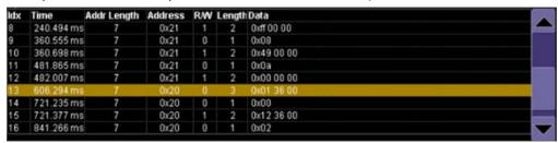
Use the vertical scroll bar on the right to navigate the protocol table. If your vertical scroll bar is yellow, the **Adjust** knob on your oscilloscope's front panel can also be used to navigate the table.
