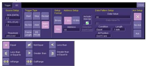
Selection of Trigger Type results in dynamic changes to the I<sup>2</sup>Cbus Trigger dialog. Simple I<sup>2</sup>C triggers, such as Start, Stop, ReStart, and NoAck, require no additional setup, while frame-based triggers, such as ADDR, ADDR+DATA, FRAME LENGTH, and EEPROM require addition user-defined setup information.
