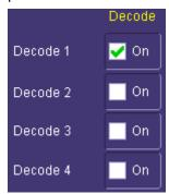
2. **Decode ON Checkbox** - If checked, it means the decoder is turned ON and decodes (provided the protocol is correctly setup in the Decode Setup dialog box).
