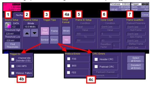
All Trigger Setups use Source Setup, FlexRay Setup, and Trigger Type fields.
