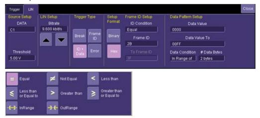
The Source Setup information must be defined. The datasheet for your part should contain the information you need to properly setup the LINbus Trigger.
