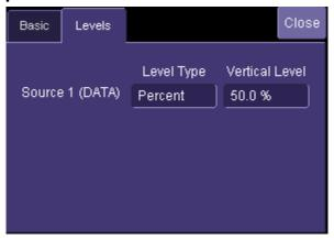
Source 1 (DATA) **Level Type** and **Vertical Level** - The message decoding algorithm setup is performed here. The level is normally set up in %, and defaults to 50%. Adjust the level by touching inside the field and highlight the box title in yellow, then use the oscilloscope front panel **Adjust** knob to make the change. Alternatively, touch inside the field twice and select a value using the pop-up numeric keypad.
