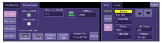
This is a single tab with an indicator on the left side describing to which of the four decoders the setup information pertains.
