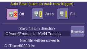
As the previous screen-shot shows, you can disable the Auto Save function by clicking the OFF button. Or, select WRAP where Auto Save occurs until the hard drive is filled, and then discards the oldest data in order to write the newest data. Lastly, select FILL which Auto Saves until the hard drive is filled and then stops.
