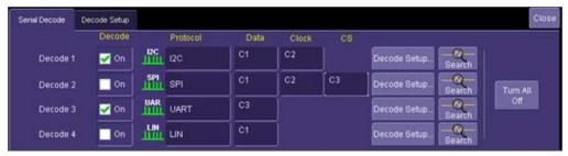
**Note**: This (previous) dialog box reflects an oscilloscope with the I<sup>2</sup>C, SPI, UART and LIN options.
