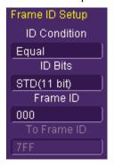
When CANbus trigger selections are either Remote or Data, use the Frame ID Setup fields as follows:
