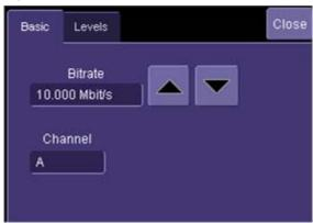
• **Bitrate** - Adjust this bitrate value to match the one on the bus to which you are connected. This bit rate selection is dynamically linked to the decoding bitrate (they are always the same value). Use the arrows to move through standard bitrates (2.5, 5.0 or 10.0 Mb/s) and make a selection. Or, touch the number twice (with a finger, or using a mouse) and open the pop-up keypad to enter the value directly.
