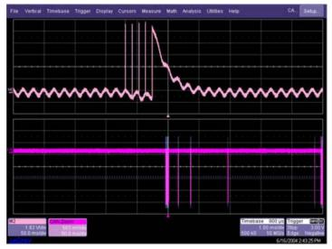
This data was acquired over a 500 ms duration. It is likely you want to understand whether the analog signal input to your electronic control unit (ECU) is creating the desired CAN message output from the ECU. There are a few ways this can be done as the following topics explain.
