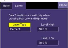
The message decoding algorithm setup is based on these field values. FlexRay is a tri-level signal and requires 2 levels for the oscilloscope to distinguish between 1 and 0. The **Level Type** is normally set up as Percent, and defaults to 70% and 30% **Level High** and **Low** values, respectively.
