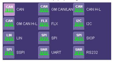
**Note**: SIOP and SSPI are part of the SPIbus TD package. RS232 is part of the UART-RS232bus TD package.
