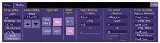
The Source Setup information must be defined. The datasheet for your part should contain the information you need to properly setup the FlexRay Trigger.
