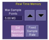
• If you choose to **Set Maximum Memory**, you can decrease the memory usage so you do not sample at too high a sample rate (too high a sample rate slows down the decoding algorithm). Then, adjust your timebase setting to a length sufficient to capture the event.
