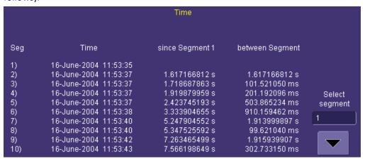
**Note**: Ten timestamps fit on the display at one time. Choose which segments to display by using the **Select Segment** control. You can also page through the segments one at a time by using the **Adjust** knob on the front panel.
