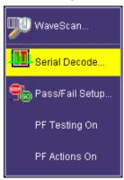
2. **Decode Protocol Selections** - As serial decode options are added to your oscilloscope, additional protocol selections are available in a pop-up dialog box within the Serial Decode dialog boxes.
